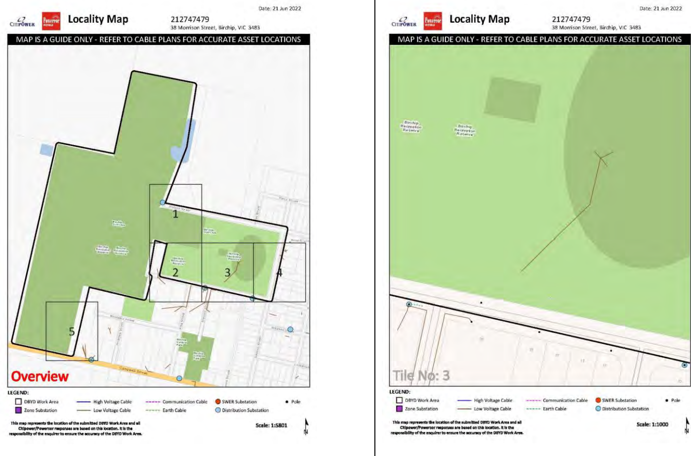
Figure 23. Site Locality Map for electrical cables at Birchip Recreation Reserve and location of low voltage cable at Oval Source: Dial Before You Dig
