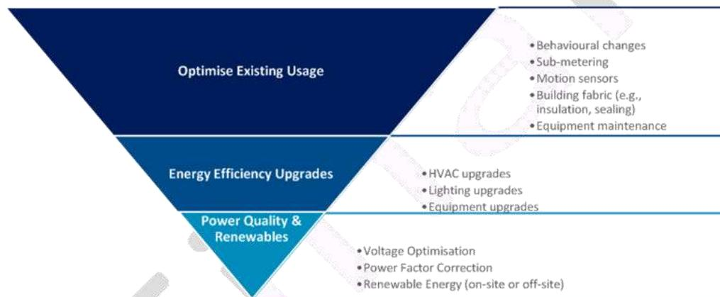
Figure 15: Energy Efficiency Hierarchy
