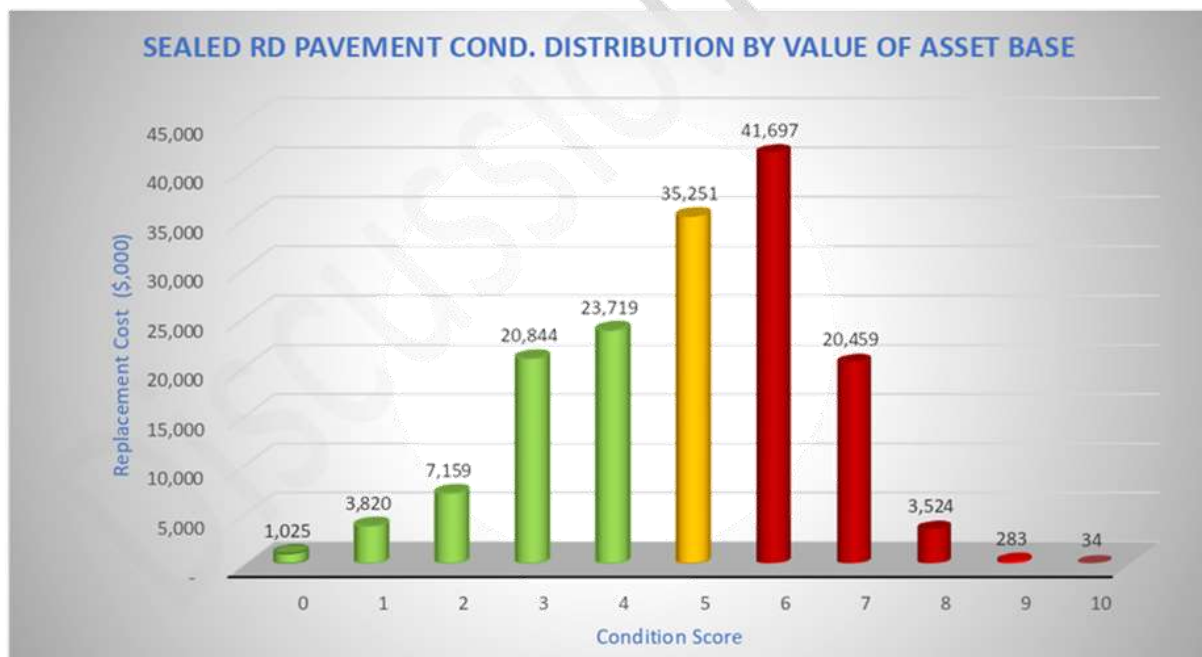
Figure 4 – Condition Profile – Sealed Pavements
