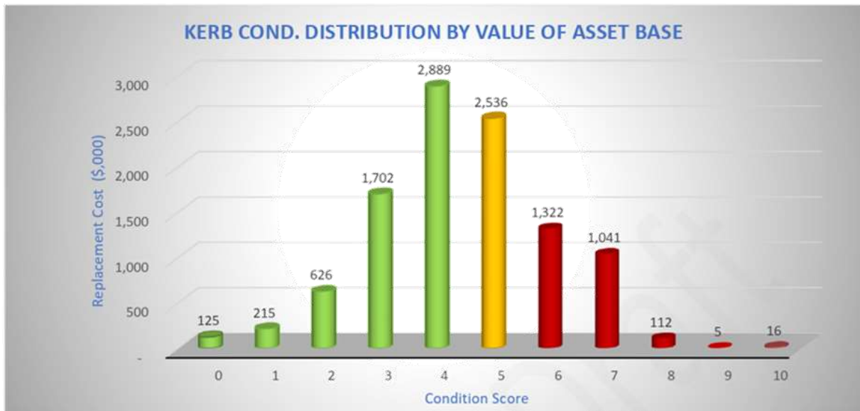
Figure 7 – Condition Profile – Kerb and Channel
